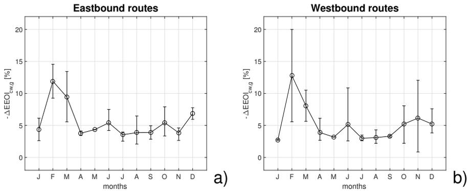
**Figure 2.** Seasonal variability of EEOI relative change of the optimal route accounting for both ocean currents and waves with respect to the geodetic route. Eastbound and Westbound routes are considered in panel a) and b) respectively. For each calendar month, the empty circle position is the mean and the error bars span between minimum and maximum value of the (four) routes pertaining to that month.
