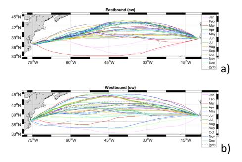
**Figure 1.** Spatial variability of the transatlantic crossings optimised considering both ocean currents and wave heights. Panels a,b) for East- and Westbound crossings respectively. The geodetic (or: least-distance) route is displayed as a black dashed line.
