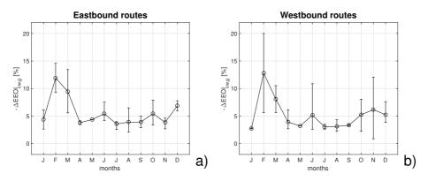
**Figure 2.** Seasonal variability of EEOI relative change of the optimal route accounting for both ocean currents and waves with respect to the geodetic route. Eastbound and Westbound routes are considered in panel a) and b) respectively. For each calendar month, the empty circle position is the mean and the error bars span between minimum and maximum value of the (four) routes pertaining to that month.
